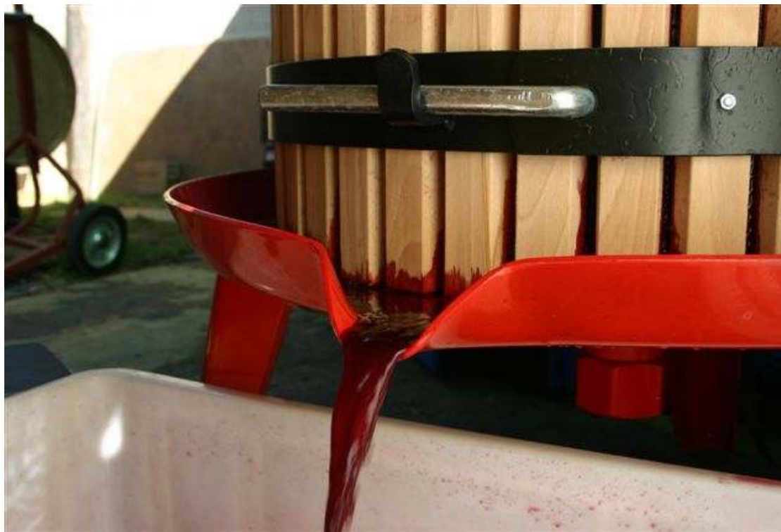
First juices flowing from the basket press, which is operated by hand
